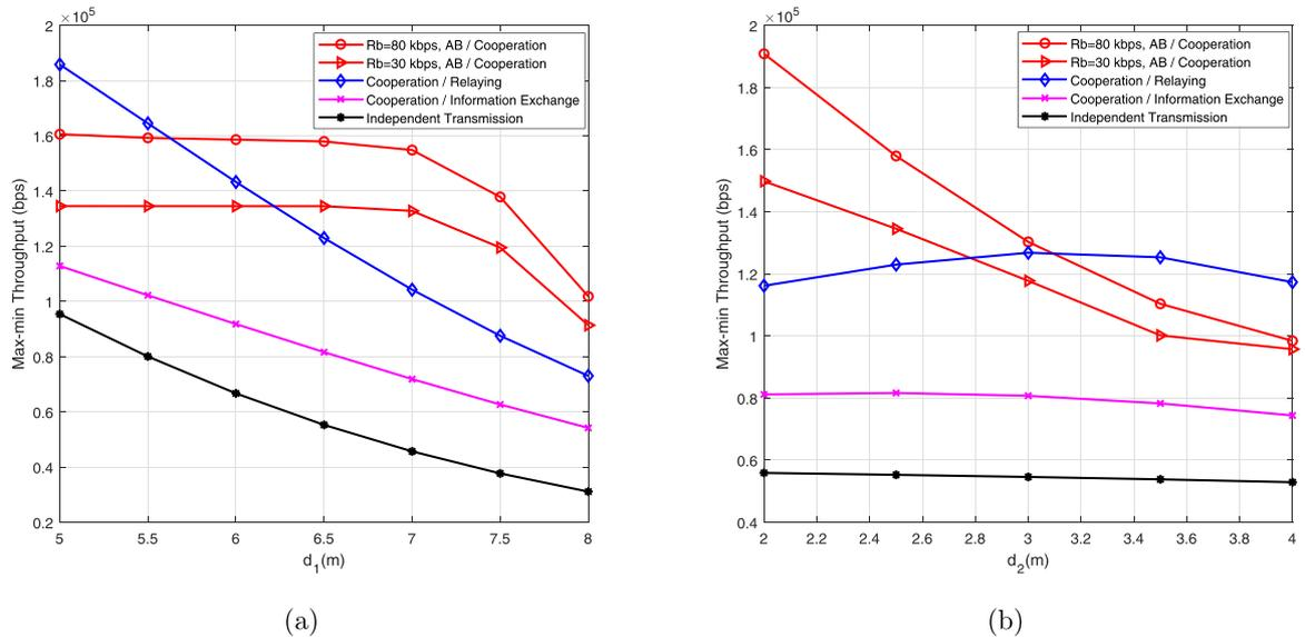
**Fig. 5.** (a) The max-min throughput performance when the inter-user channel  $h_{12}$  varies. Here, we keep  $d_2 = 2.5$  m and vary  $d_1$ . (b) The max-min throughput performance when the relaying channel  $h_2$  varies. Here, we keep  $d_1 = 6.5$  m and vary  $d_2$ .
