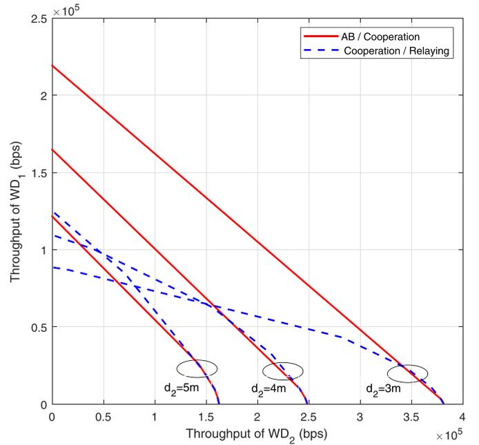
Fig. 7. Throughput region comparison of different methods.
